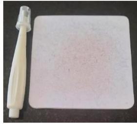
**Figure 15:** A picture of a leaf puncher and mat used for making leaf discs.
