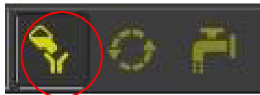
Figure 6. Icons for Prime (highlighted for use during priming), work, and clean mode.
