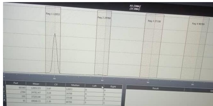
Figure 13. Peak at absorbance frequency 200 in region 1 indicating well calibrated machine.
