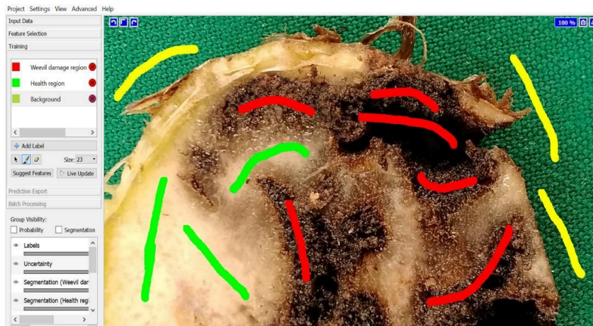
Figure 5: Training Ilastik by selecting label and annotating corresponding area (red: weevil damage, green: intact corm areas, yellow: background)
