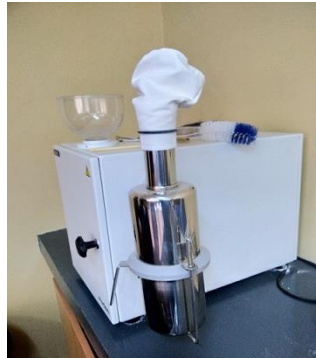
Figure 2. Labconco laboratory milling machine ( to grind samples to fine particle size)
